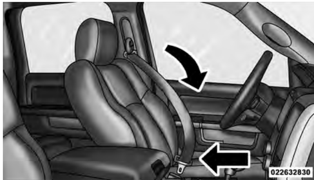
Pulling Out Latch Plate And Webbing
